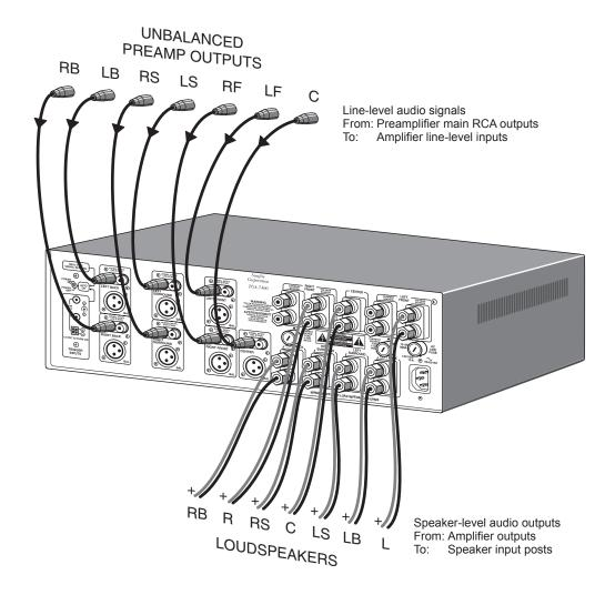
If your preamplifier has RCA outputs, it can be connected to the amplifier inputs as shown. The amplifier will boost the preamplifier's output, up to a level suitable for driving speakers.
